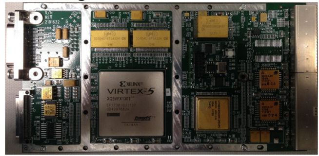
Figure 2 - LIDAR High-Speed Digitizer Card
