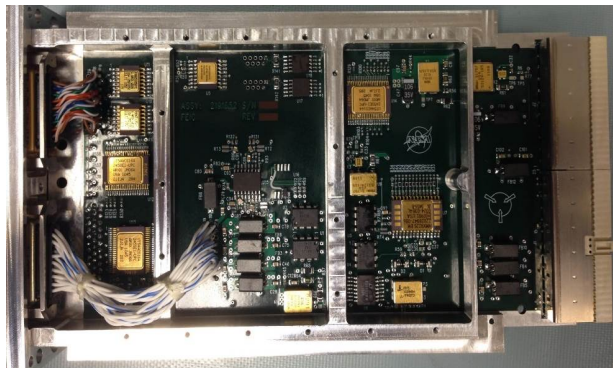
Figure 4 – LIDAR Front-End Interface Card
